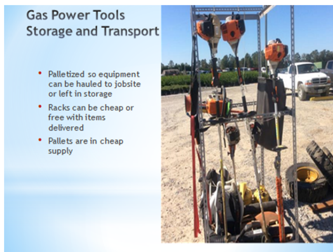
Figure 4. Gas powered tools are stored and transported with racks attached to pallets.
