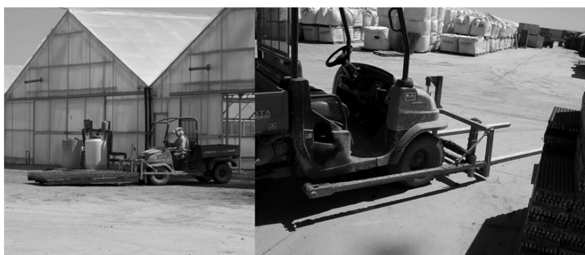
Figure 2. A homemade fork system that has been used to move plants at a nursery in California for about 20 years.
