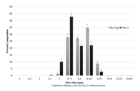
Figure 4. Differential distribution of medium sand measured by Ro-Tap and CPA-2.
