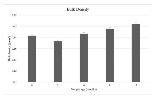
Figure 3. Bulk density of pine bark sampled at five different ages (0, 3, 6, 9, and 12 months) determined using the NCSU porometer method.
