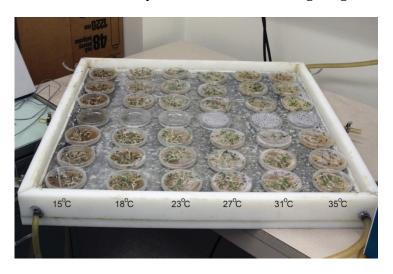
Figure 1. Thermogradient table.
