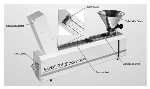
Figure 1. Tyler (Haver) computer particle analyzer 2 conveyor.
