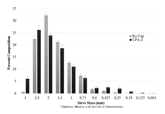
Figure 3. Differential distribution of coarse sand measured by Ro-Tap and CPA-2.
