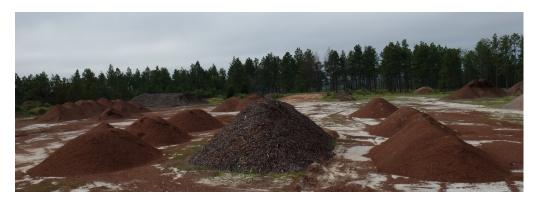
Figure 1. The long term, commercial scale pine bark aging study located at T.H. Blue, Inc., Eagle Springs, North Carolina. Pine bark fines (5/8 in.) were placed in three pile replications and aged for 12 months.
