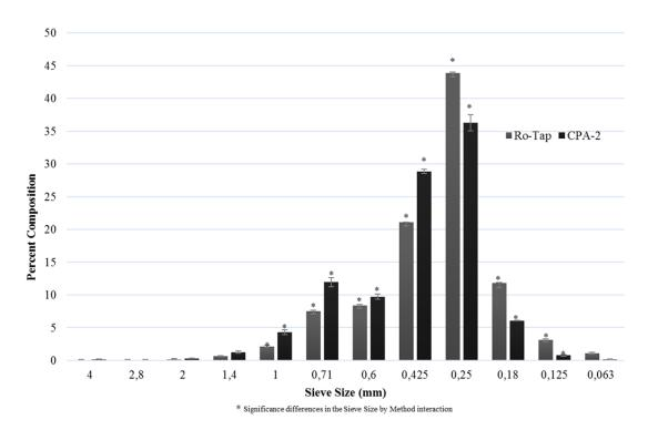
Figure 5. Differential distribution of fine sand measured by Ro-Tap and CPA-2.
