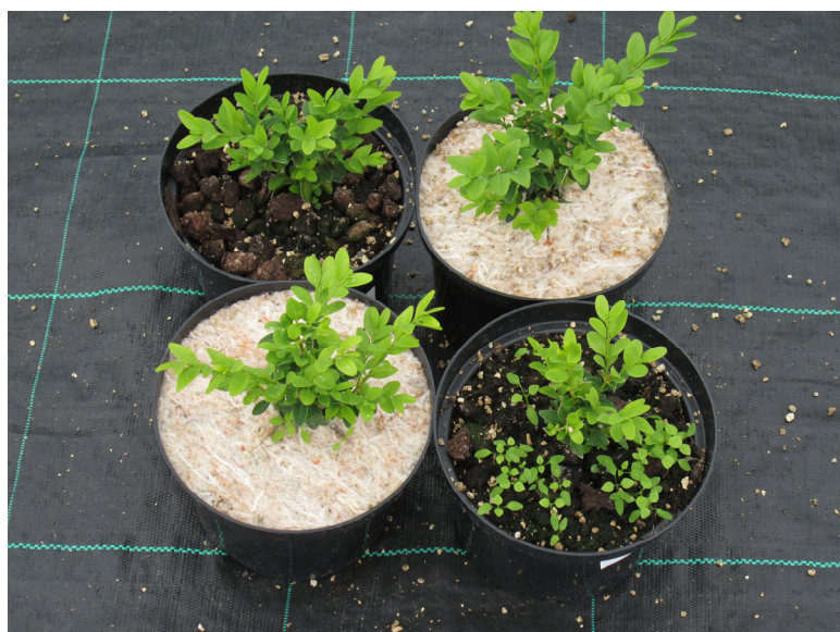
Fig. 3. Weed growth in pots with and without recycled wool fabric mulch discs (pot top left was unseeded).
