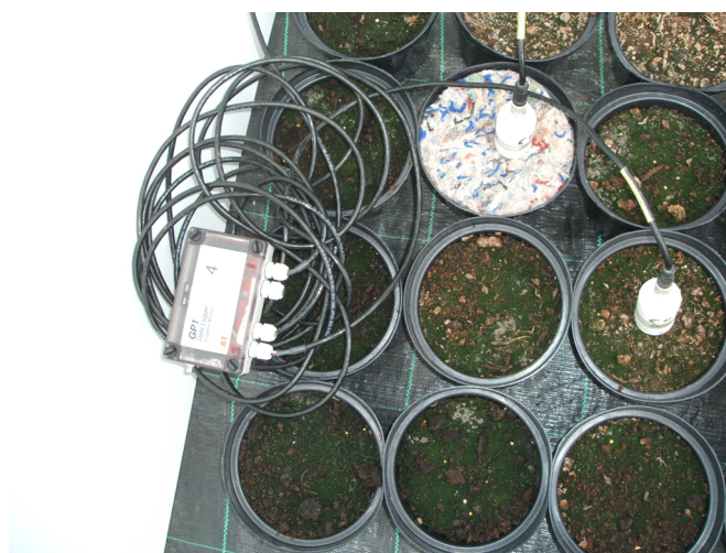
Fig. 4. Delta T moisture and temperature measurement equipment in place. Probes inserted in pot with pot cover and pot without pot cover.
