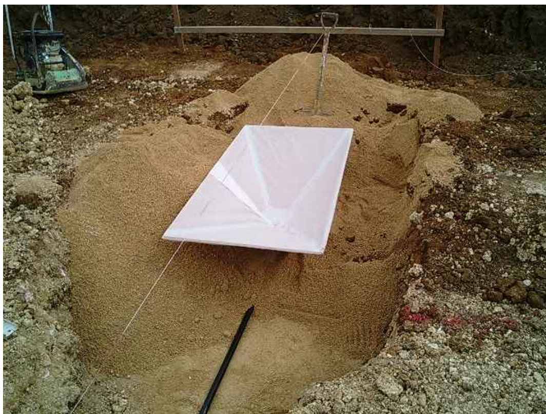
Fig. 1. The Rohto-type lysimeter was buried 60 cm depth in the sugarcane field.
