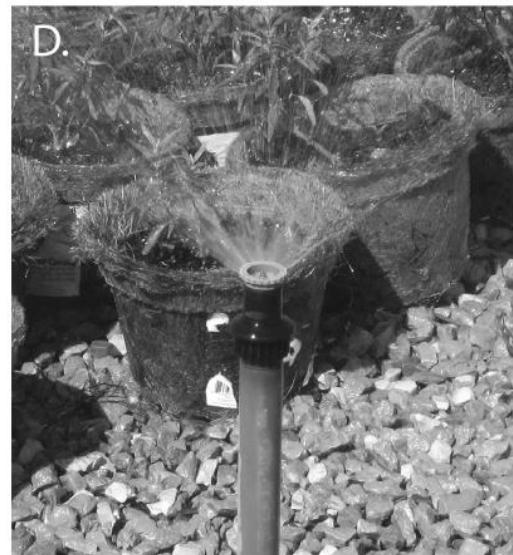
Fig. 1. (A) Sprinkler head types; (B) Rotary impact head sprinkler; (C). Rotary spinning head sprinklers; and (D) Stationary head nozzle.
