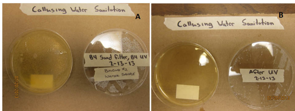
Figure 4. (A) Water inflow to callusing filtration system showing high levels of bacterial contamination; (B) Water outflow from the filtering system to the callusing baths with no biologicals present.
