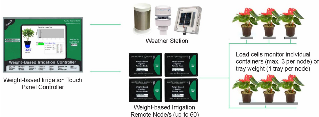
Fig. 2. Components of weight based irrigation controller.
