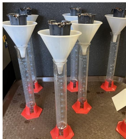
Figure 2. Modified NCSU porometer method using individual 1-inch cells for determining air space, container capacity, and bulk density.
