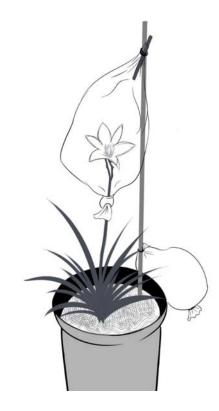
Figure 1. Schematic diagram of the collection system. The column containing the adsorbent polymer is attached to the upper part of the stake, and an empty bag, from which volatiles were sampled to account for background contaminants, is attached to the lower portion of the stake.
