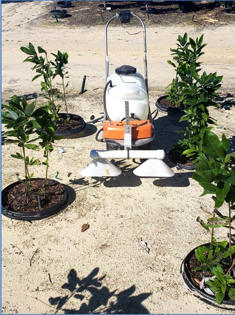
Figure 1. Jacto PJB16 battery powered backpack. Used for watering in granular herbicide applied to pot-n-pot containers.
