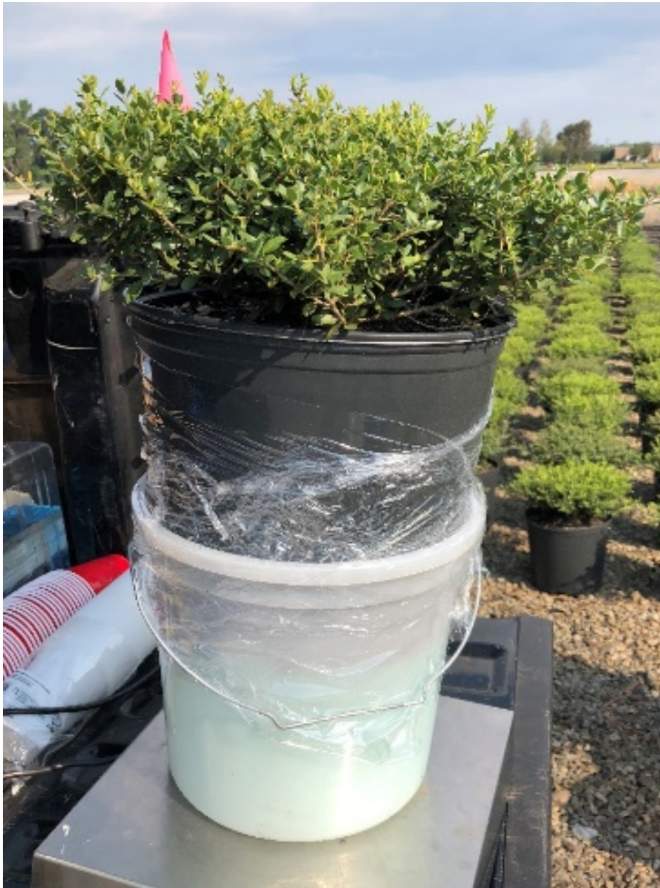
Figure 2: "Skirted" sample for irrigation efficiency analysis
