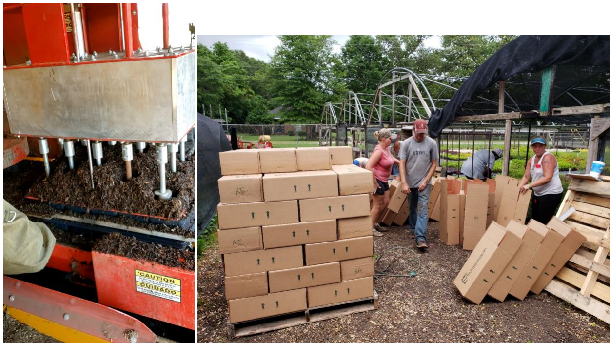
Figure 9. (left) Ellis Manufacturing to build a 15-bit drill-head for our potting machine capable of producing jumbo quarts. (right) We can box and palletize the quarts to ship with our liners.
