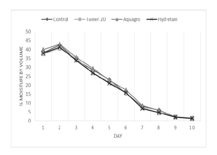
Fig, 3. Soil moisture content (SMC) measured as % water by volume. Measurements taken at 7:00 daily for ten days. SMC was measured with a Delta T HH2 soil moisture sensor (Delta T Devices).
