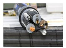
Fig. 1. A multiprobe Sonde set to continuously monitor water quality
