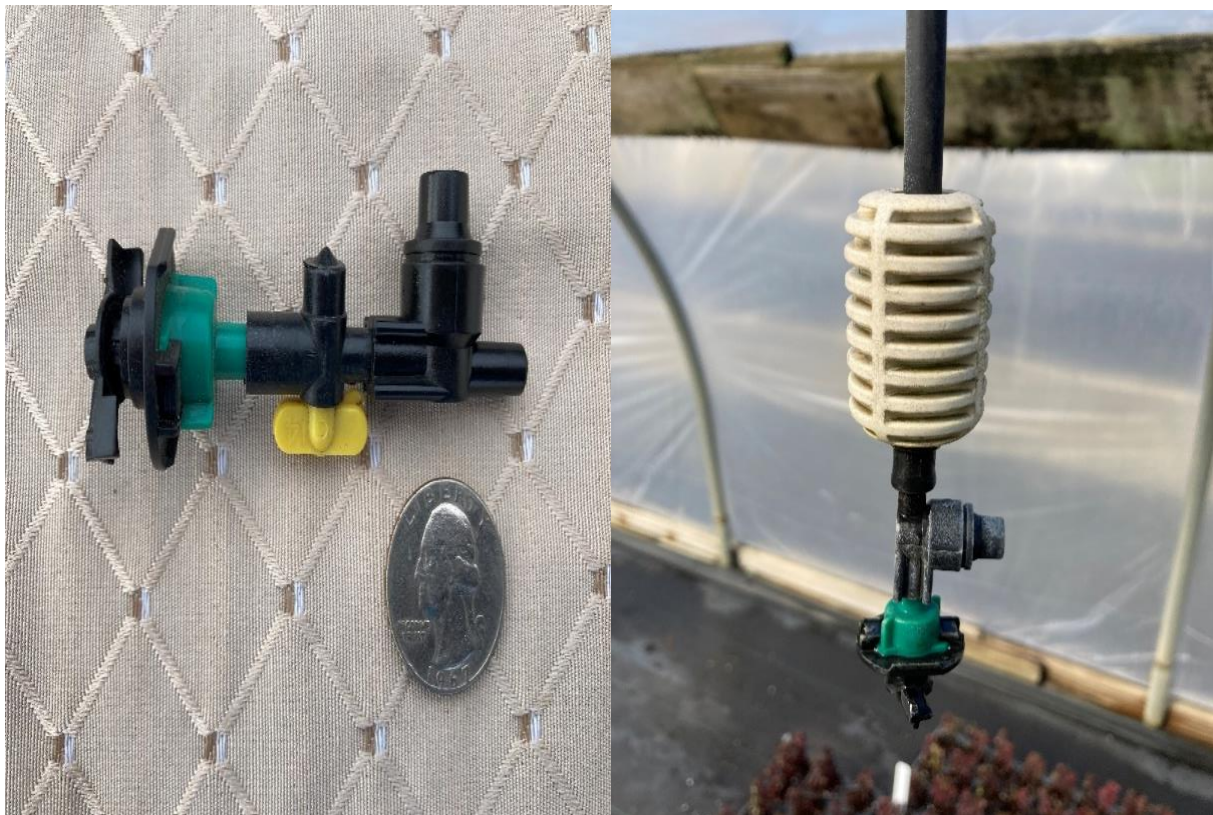
Figure 16. (Top, bottom left) Mini-Sprinklers are manufactured by Tavlit®. They are the 866 mini-compact sprinklers and can accommodate a variety of color-coded spinners which have different flow-rates. (Bottom right) An anti-drip device is included in the design to quickly discontinue the misting event.
