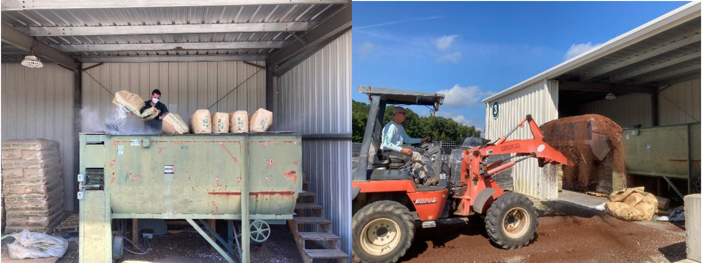
Figure 9. (left) Loading coarse perlite into 3.8 m 3 (5 yd 3 ) paddle mixer, and (right) loading bulk aged loblolly pine bark into the paddle mixer.
